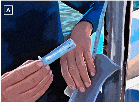
Figure 5. Subsampling of the core using a 25 mL cut-off polyethylene syringe. The duct tape is peeled back starting at the top of the core (A); the syringe is used to remove a sediment sample from the core (B,C); the exact volume of sediment within the syringe is noted on a datasheet (D) before transferring the subsample into a pre-weighed glass vial.
