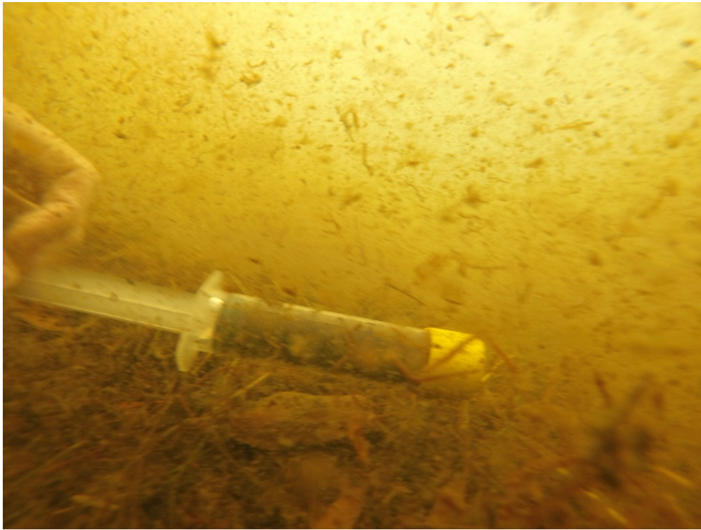
Figure 4.2: Unstable, low-density sediments of impaired canals can easily be disturbed. Note the dead leaves and plant detritus that dominate surface sediments rather than expected sand grains. The pictured device was used to remove cores of surface sediment for laboratory analysis.
